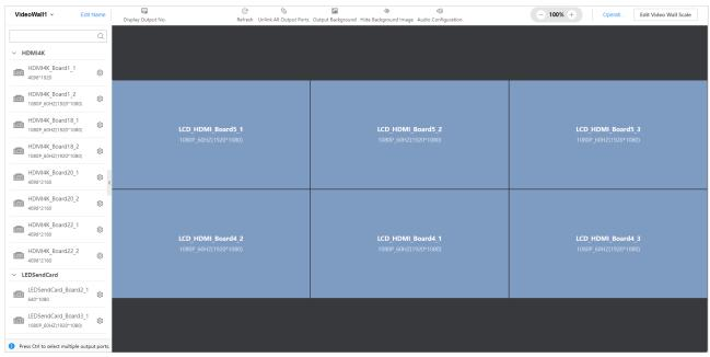
Figure 3-28 Bind Output Ports with Video Wall
