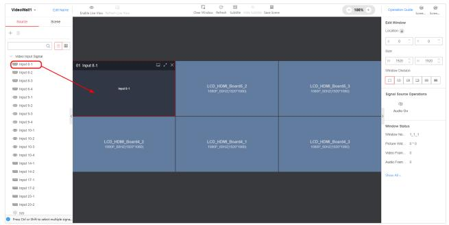
Figure 3-33 Bind a Signal Source to LCD Video Wall
