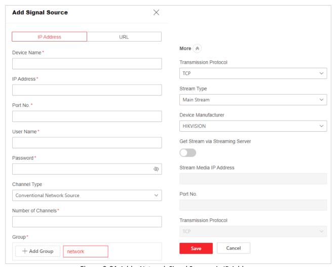
Figure 3-31 Add a Network Signal Source via IP Address
